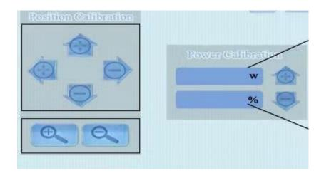
Power calibration: selected , Select the power value to be calibrated, and then select , Adjust this value and use the laser power meter to measure the actual power of the laser at this time, so that "display value of power to be calibrated" = "laser maximum power" × "percentage of actual power to be calibrated", please save it before exiting.
