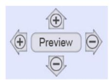
Use the up and down plus and minus buttons to adjust the maximum length of the dot pattern in the up and down direction to 0-20mm.
