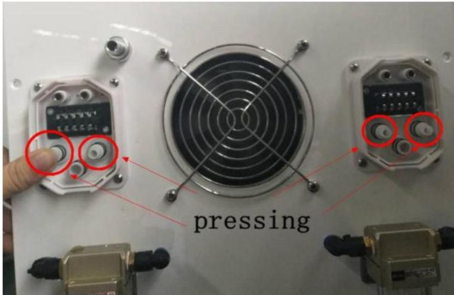
**Thirdly:** Turn off machine and connect the cryo handle (**Note:** The cryo handle must be placed below the freezer connection, allowing water to flow smoothly into the handle)
